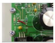
Before re-installing the circuit board into the case, replaced the original display standoffs with the four shorter ones provided in the kit.
