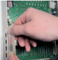
Remove 4 screws holding circuit board and pull the board out of the case
