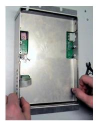
• Plug 3 Pin connector into new Dixmor display (Connector is keyed and should slide in with little force)
